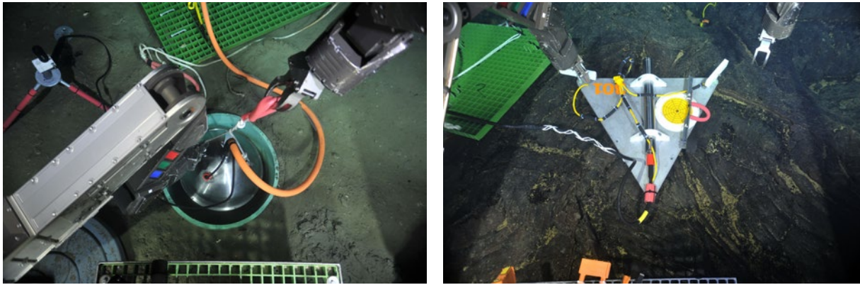
Figure 9. (left) A broadband OBS installed in a caisson that will be filled with silica beads to dampen noise yet provide good coupling to seabed ground motion. (right) A short-period OBS installed at ASHES vent field on Axial Seamount. The sensing unit is housed in titanium to resist corrosion. (Photos from NSF-OOI/UW/CSSF.)
