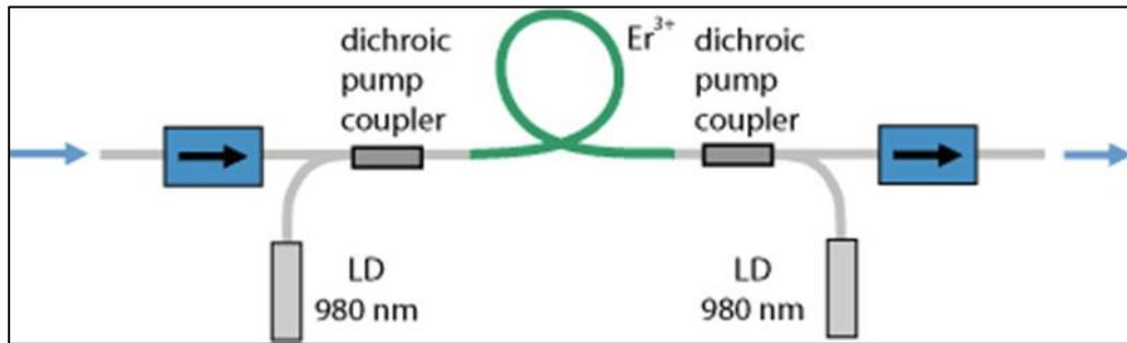
**Figure 3. Basic optical amplifier (image from rp-photonics.com<sup>14</sup>)**
