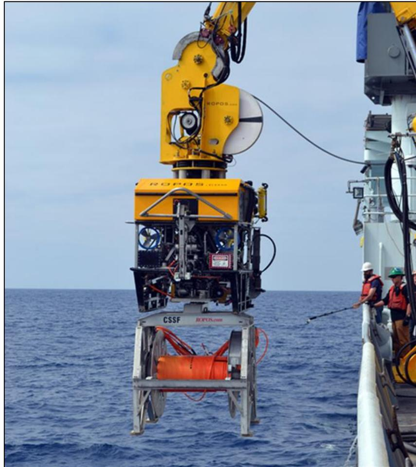
**Figure 10. ROV preparing to deploy a secondary cable on the OOI-CA**
