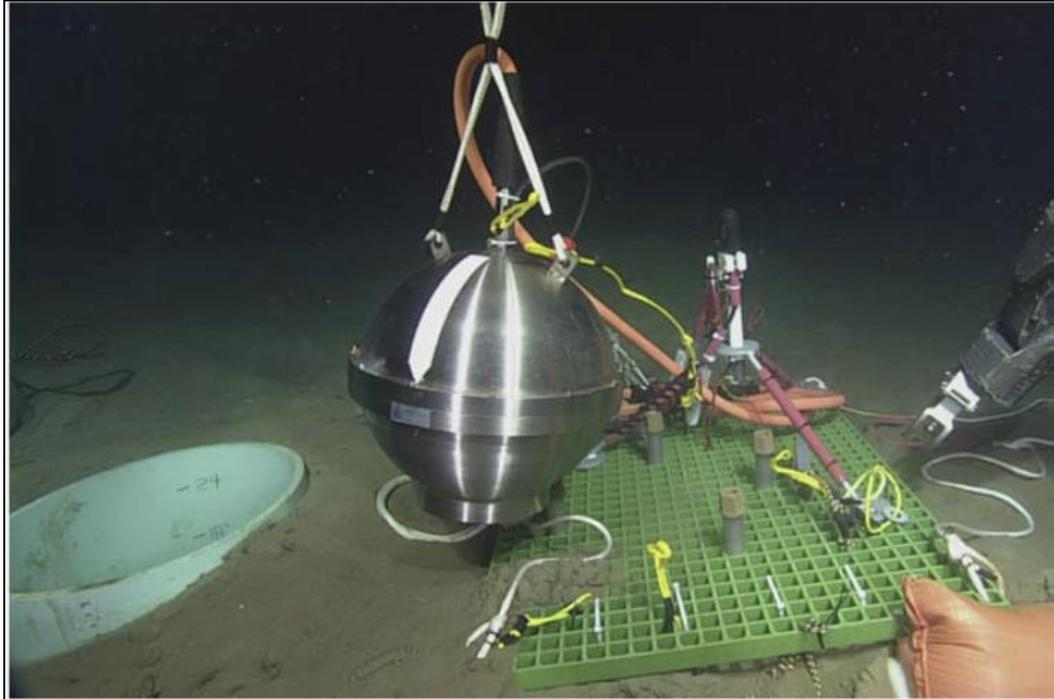
**Figure 16. Güralp broadband OBS installation by ROV on the OOI-CA**
