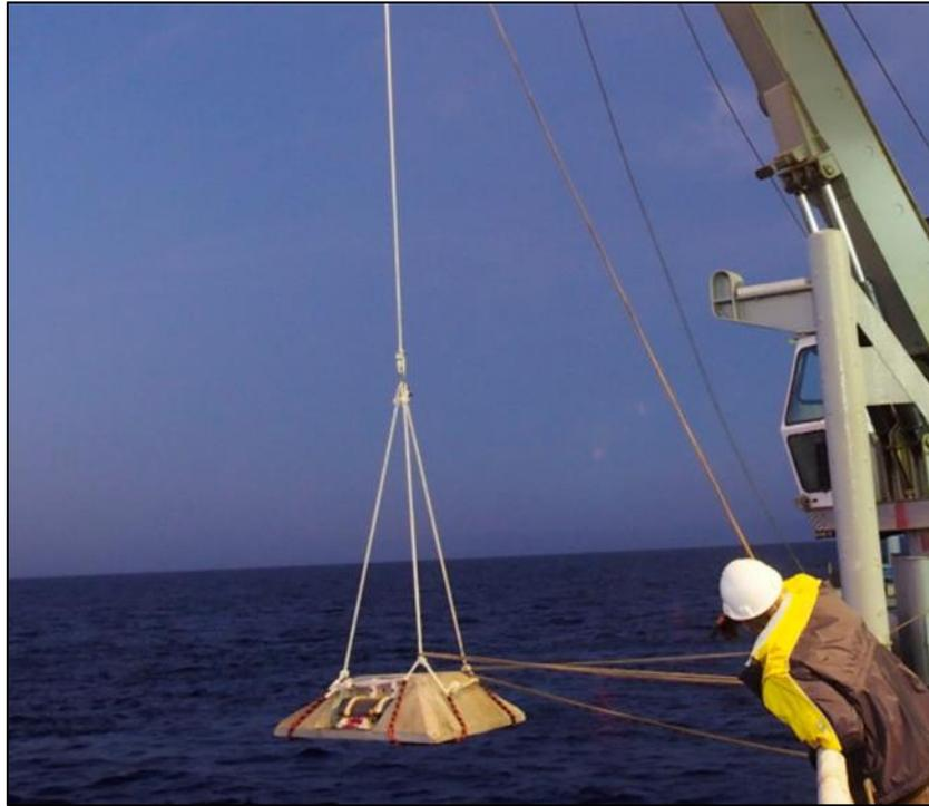
**Figure 17. Custom BPR Secured to Concrete Monument Being Installed on the OOI-CA**
