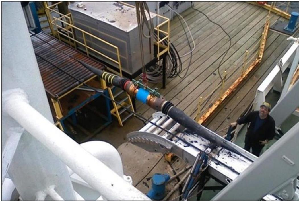
**Figure 5. Repeater being loaded onto C/S Dependable in preparation for deployment onto OOI Cabled Array<sup>17</sup>**
