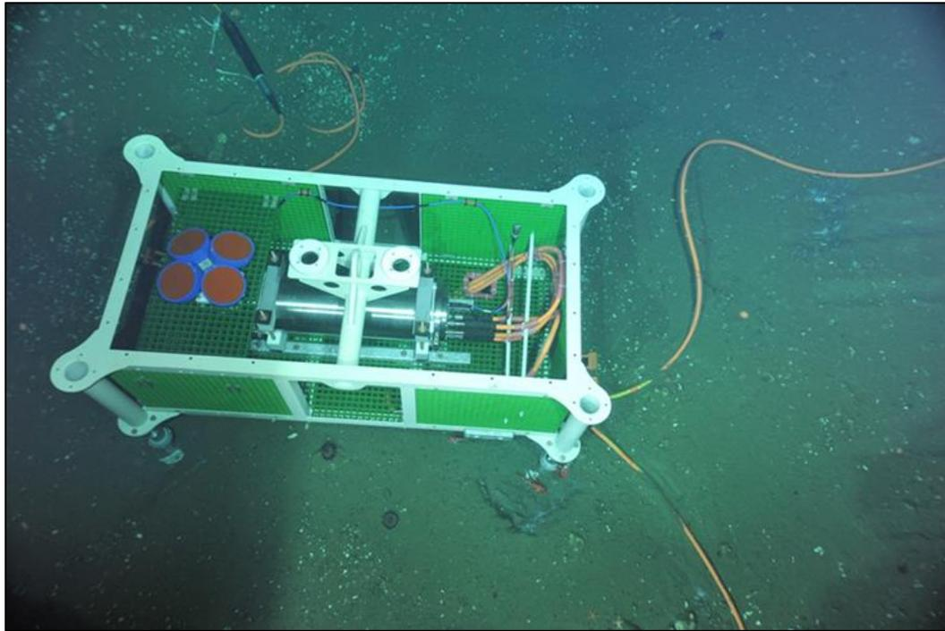
Figure 7. OOI-CA junction box on the seafloor
