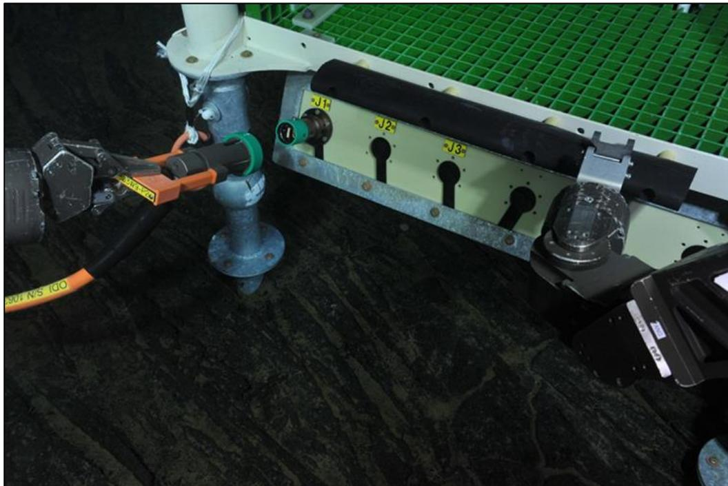
Figure 8. ROV connecting a wet-mate connector to an OOI-CA junction box
