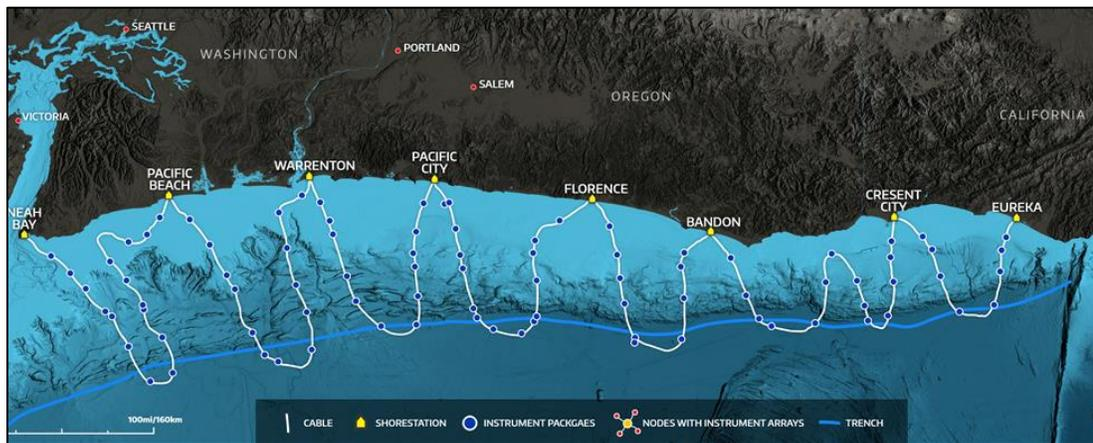
**Figure 1. Conceptual configuration of a cabled Cascadia EWS**
