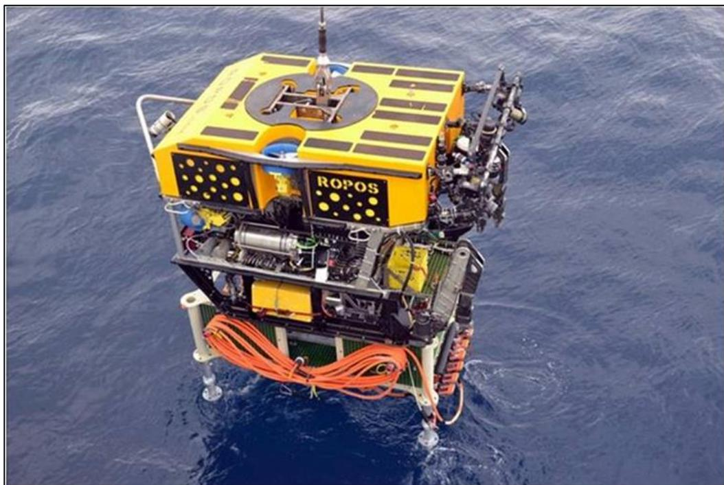
**Figure 9. ROV with junction box being lowered for installation on the OOI-CA**
