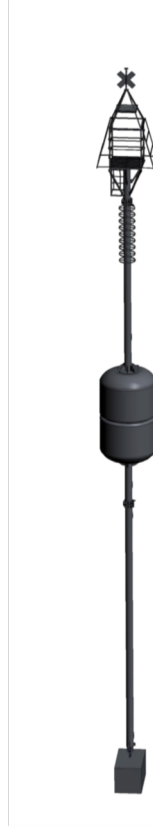
Figure 3. Sketch of buoy, showing ballast (base), float (center) and superstructure (top) with GPS, batteries, and solar panels. Water-line is between float and superstructure. Ballast and float are scaled to water depth.
