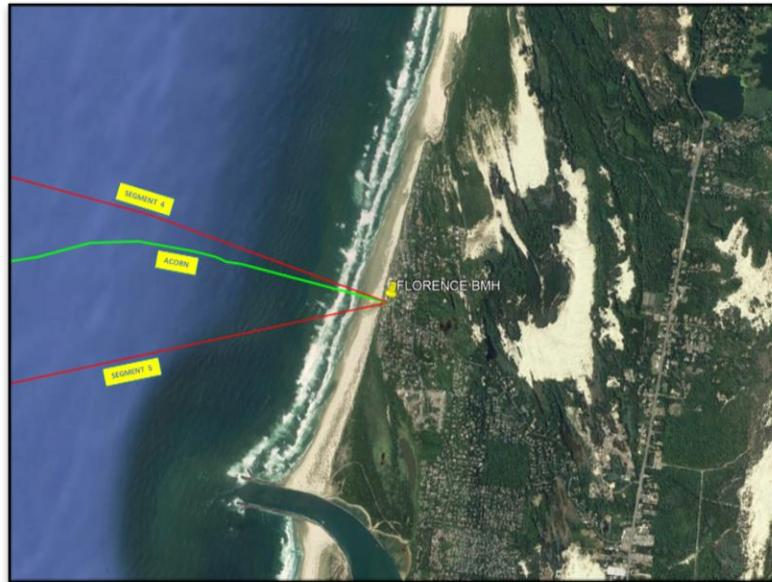
Figure 13.5-1 Segment 5 Cable Landing
